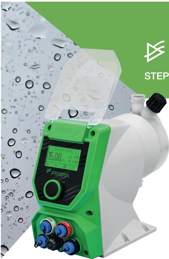
The PRISMA diaphragm and stepper motor metering pump is designed for applications requiring high precision dosing volumes and reliable repeatability. Thanks to the microprocessor controlled stepper motor and excellent pitch resolution of 1: 4800, the entire stroke and suction cycle is controlled with maximum precision. Maximum stroke frequency: 175 st/m.
